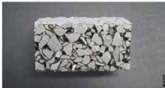
Figure 1 – Solar Heat-blocking Pavement
